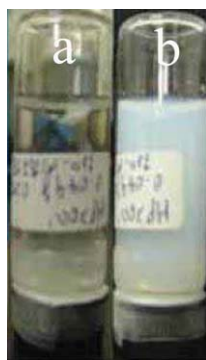
Figure 3 The snapshot of the highly branched PNIPAN HP20 after aminolysis without oxidation in aqueous solution at 20°C (a) and 36°C (b). The concentration of polymer in water is 25 wt %. [Color figure can be viewed in the online issue, which is available at www.interscience.wiley.com .]
